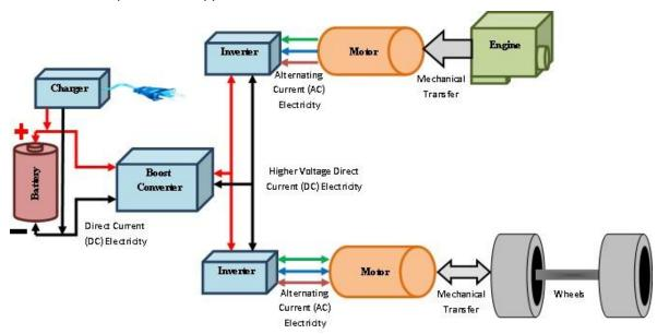
Figure 3: An Electrical Car System (www.electricdrive.org)
