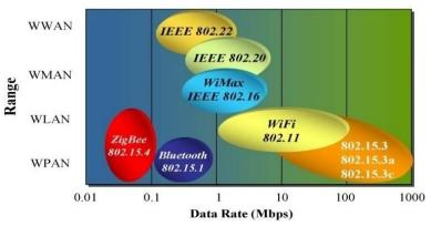
Fig. 1. The 802 wireless spaces a graphical comparison
