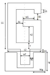
GEOMETRY OF THE VARIOUS DESIGN PARAMETERS OF THE PROPOSED Measurement Parameters in mm h1 1.2 10 g1 10 w1 S1 3.3 h2 10 Т 3 h3 4.69 g2 1.35
