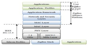
Fig. 2. The ZigBee Standard and IEEE 802.15.4
